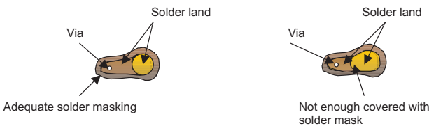
Figure 14. An example of adequate and inadequate solder lands potentially affecting the height of the BGA.
